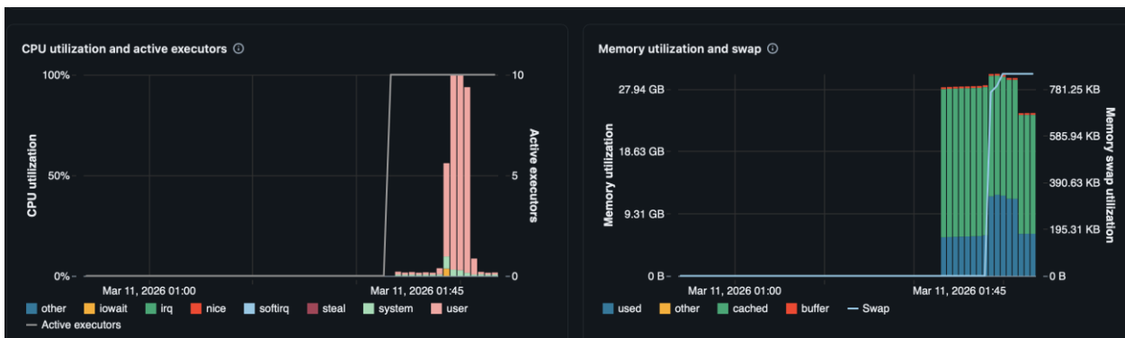
CPU Utilization and Memory Utilization Of All Executor Nodes In Spark Only Cluster
