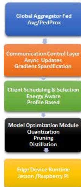
Figure 2: Multi-Layer Optimization Framework for Federated Learning on Edge Devices
